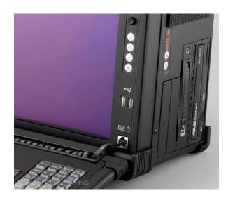
The EMP-370 is a rugged workstation based on a fully customizable aluminum chassis with ample space for adapters and five full size bays that lets you bring to field the power of a state-of-the-art workstation. Its drive bays can be custom fitted with standard 5.25 computer peripherals like Tape Drives, Removable Disk Drives or a fix RAID.
